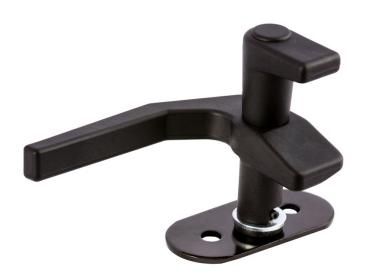
This easy to operate window handle is designed to fit comfortably in the hand for top and side hinged windows for on and off-highway vehicles. Featuring 90 degree rotation with steel mounting plate and glass filled nylon handle. Provides two position venting.
